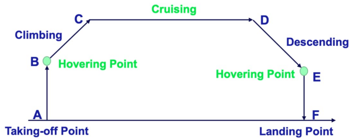
Figure 18 Flight pattern used in the energy consumption model for EH216
